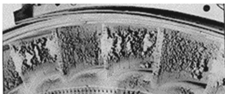
Fig. 2 Image of turbine nozzle guide vanes after ingestion of volcanic ash [3]
