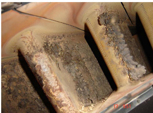
Fig. 2 Deposition on first stage vane of utility gas turbine after approximately 8000 h of service. Firing temperature 1150°C.
